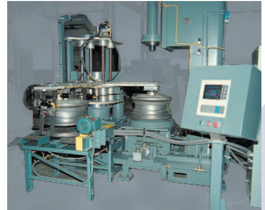
Pick-N-Place Automation 250-lb capacity, 5-ft radius
