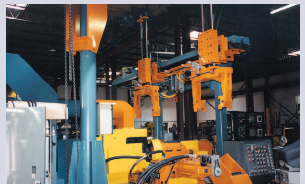
Dual Gripper 2-Axis Overhead Gantry 144" horizontal travel, 36" vertical travel
